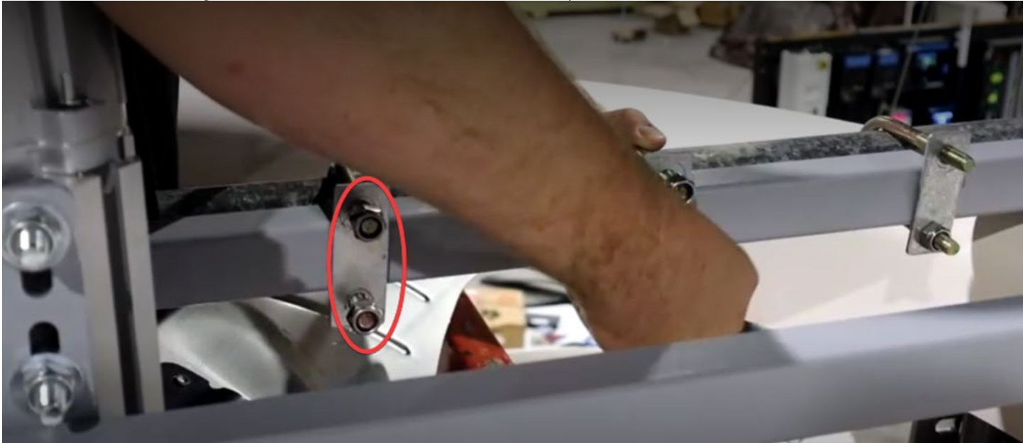
10. Thread and tighten the nuts on each end of the U-clamp.
